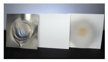
Pictured above from left to right: Aluminum panel exposed to > 1000°C flame impingement, aluminum panel coated with 0.1mm FyreWrap LiB coating (no flame impingement), aluminum panel coated with 0.1 mm FyreWrap LiB coating after being impinged by a flame > 1000°C. Test set-up shown in areater detail in picture below.
