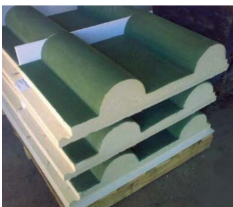
Figure 6. To withstand the severity of the furnace environment, Carbowall panels receive a mullite-based coating. This coating enables the panels to resist the high gas velocity inherent in this area, and withstand abrasion caused by soot or the velocity of steam injected to clean the pipes.
