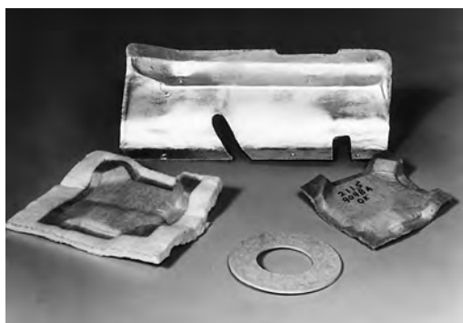
Press-formed parts made from Fiberfrax Duraset felt.
