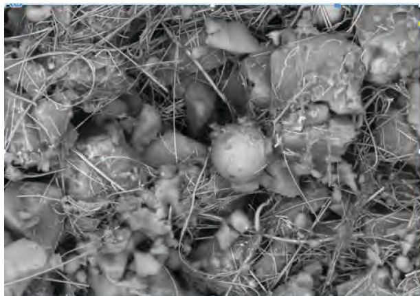
Figure 1. Microscopic SEM image of AlkeGel blanket showing aerogel particle and fibre matrix.
