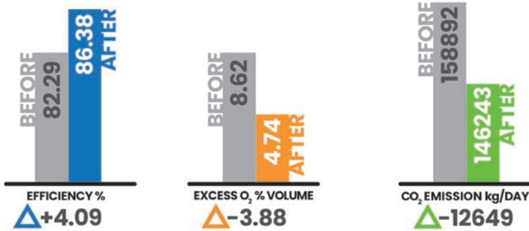
Figure 3. The actual measurements taken from the refinery show the increased energy efficiency of the equipment, including the reduction in CO 2 emissions.
