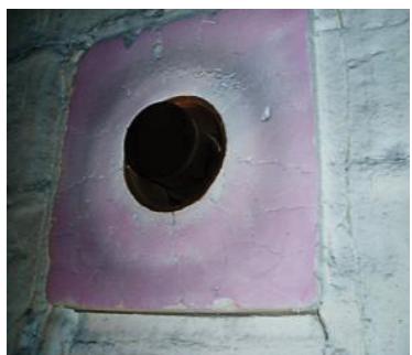
Burner Block BBM-15 7 years of use / weight: 25 kg
