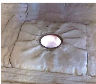
Burner Block BBM-16 17 years of use / weight: 27 kg
