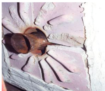
Burner Block in refractory 2 years of use / weight: 140 kg
